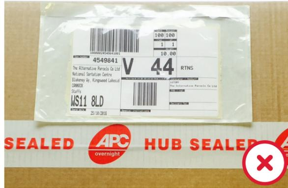
Labels should not be placed in a document holder or a plastic wallet as reflections from the plastic means that the sort scanners will not read the barcode,
